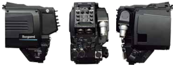
Compression free analogue HD triax Transmission Adaptor for Unicam HD.
