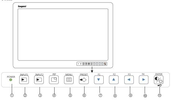
(1) Power indicator: When the power is in "ON" mode ------ Illuminate in Green
