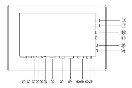
① Power switch : The power to "on", "off". ② DC input socket : Connect the AC cord.
