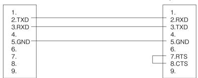
Do not connect anything to pins 1, 4, 6, 7, 8, or 9 on the monitor side (or else, a malfunction of the monitor may occur).
