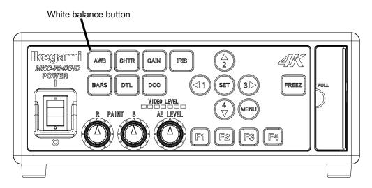
• "AWB" will appear on a monitor screen. When the adjustment is complete successfully, "AWB COMPLETED" will appear.
