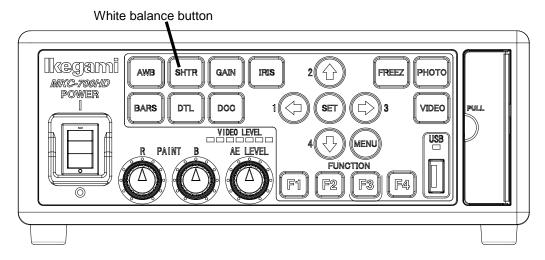
"AWB" will appear on a monitor screen. When the adjustment is complete successfully, "AWB COMPLETED" will appear.
