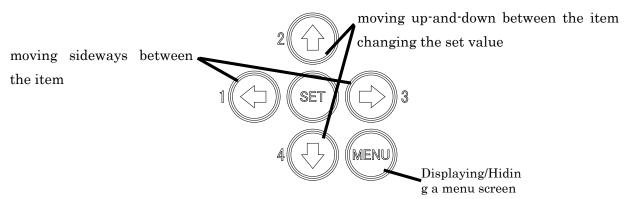
\*When, with a menu screen displayed, you press the menu button on the CCU front, the settings will be saved and the menu screen will close.
