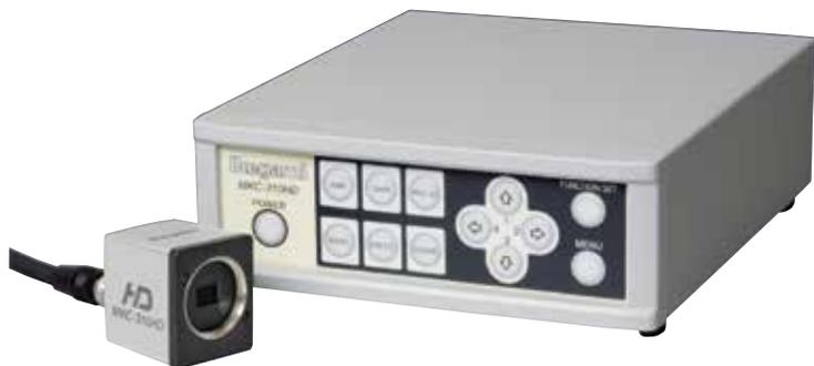
The MKC-310HD employs 3x 2.1Mega pixel Full-HD 1/3-inch CMOS Sensor to provide 1000 lines of high definition video images through 3G-SDI output interface, coupled with High Sensitivity performance of F10/2000 lux providing the optimal video quality required for special applications.
